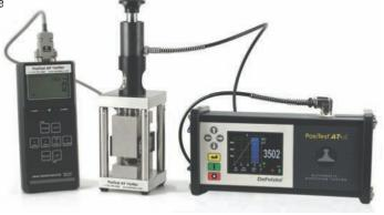
Adhesion testers include everything needed for testing: Adhesion Tester, built-in rechargeable NiMH battery with charger, dollies, abrasive pad, cutting tool, glue with mixing sticks and palettes, cotton swabs, USB cable, PosiSoft Software, instruction booklet and video, shoulder strap (AT-A only), Certificate of Calibration traceable to NIST, and sturdy, lightweight carrying case
