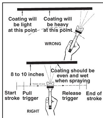
For best results, use 3 to 6 psi fluid pressure. Higher than 6 psi fluid pressure may be required for heavy-bodied materials. Low fluid pressures will produce a narrower than normal spray pattern. Generally use 30-35 psi air at gun inlet. Unusually heavy, difficult to atomize fluids may require up to 50 psi air at gun inlet.
