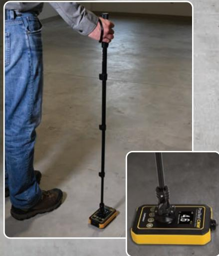
Ergonomically measure without bending or kneeling with the optional Telescopic Extender
