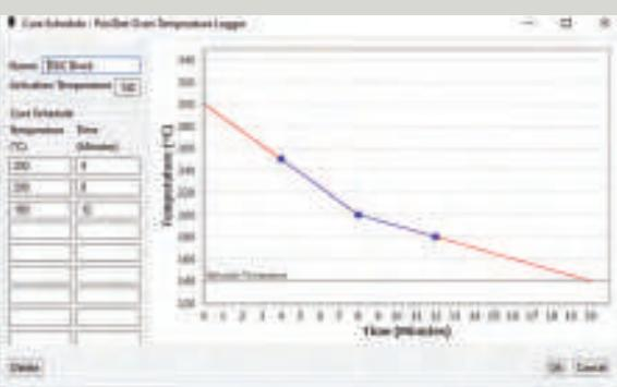
**NEW Cure Index** calculates the correct time at temperature based on supplier's cure specifications to ensure a proper cure
