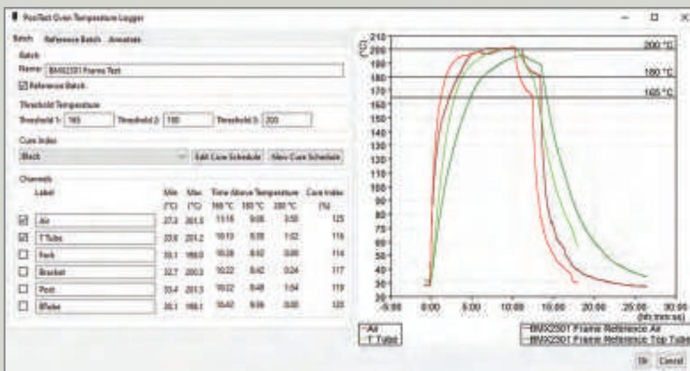
Assign names to each channel and view **Cure Index**, **Time above Temperature**, and other statistics
