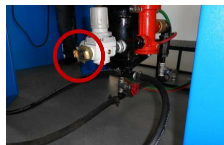
5. Connect the two 13mm to the extractor from the cabinet as per pictures. These hoses are for the vibrators and so it makes no difference to which side they are connected. Secure hoses with clamps.
